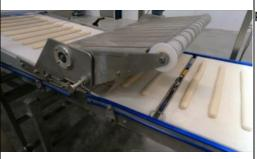
Depositing of **perfectly aligned baguettes** on peelboards
