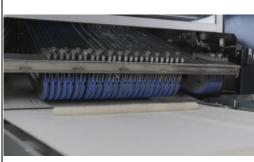
Final stretching of the product with **the cassette stretcher**, ensuring the right position of the cut products during depositing.
